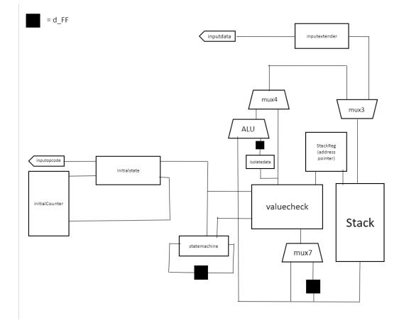
Note that this diagram excludes some registers used to acquire inputs into the valuecheck block.
