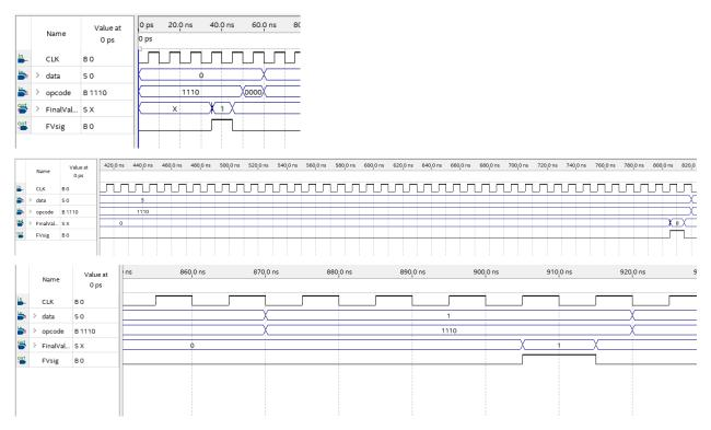
All the test results are correct and when they are calculated, the FVsig output pulses as desired.
